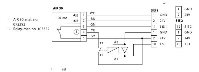
Illustration: Static condition with operating voltage switched on
