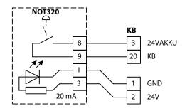
Contact sensor inside Automatic sliding doors
