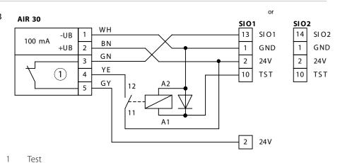
Illustration: Static condition with operating voltage switched on
