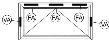
FA napęd okienne (E 9x0 L/R, E 250 NT, Slimchain, Powerchain)
