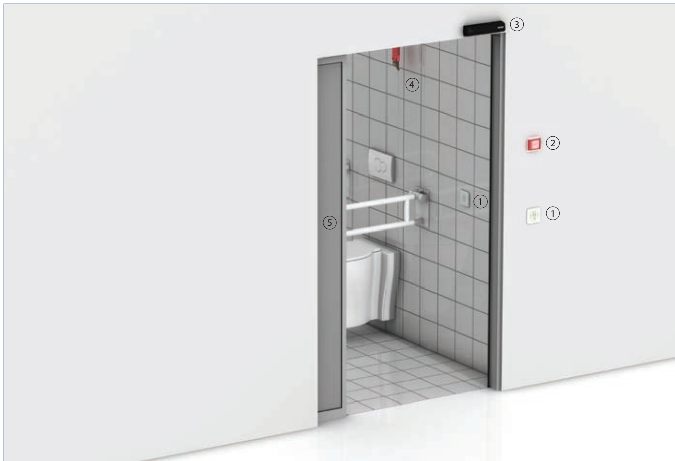
1 = Non-contact proximity switch (internal and external) | 2 = emergency off switch (recommended installation height: 1600 mm) | 3 = active infrared light curtain | 4 = emergency call pull switch | 5 = sliding panel
