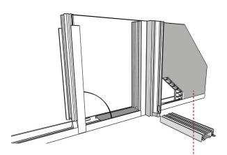
2 plasterboards (13mm) or 2 chipboards (12 or 15mm) + 85mm acoustic insulation Finishes: Melamine faced, laminated, vinyl or metal sheet
