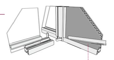
2 coated plasterboards (13mm) or 2 melamine faced chipboards (12 to 16mm) + 30mm acoustic insulation Finishes: melamine faced, laminated, vinyl or metal sheet
