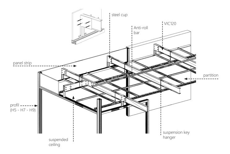
Details view - CEILING WITH GIRDERING (top view)
