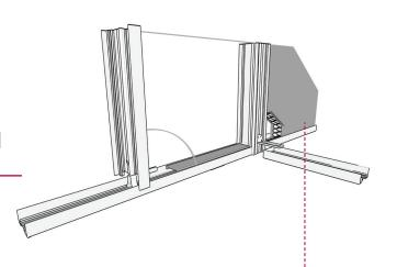
2 plasterboards (13mm) or 2 chipboards (12mm) + 45 or 60mm acoustic insulation Finishes: Melamine faced, laminated, vinyl or metal sheet
