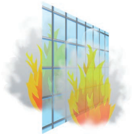
Fire from any side. Infill wall, max. height 3000 mm.
